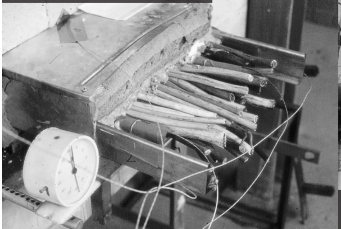
Test set-up for the first OBO cable insulation
