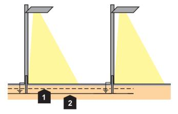
Cable routing and earthing on the luminaire mast
