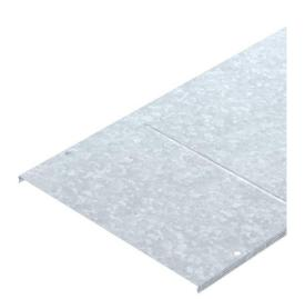
Lockable cover for mesh cable trays of type GR and GRM. Protects cables from damage, contamination and moisture from above. Suitable for industrial areas such as mechanical engineering. With transverse bead from 400 mm width.
